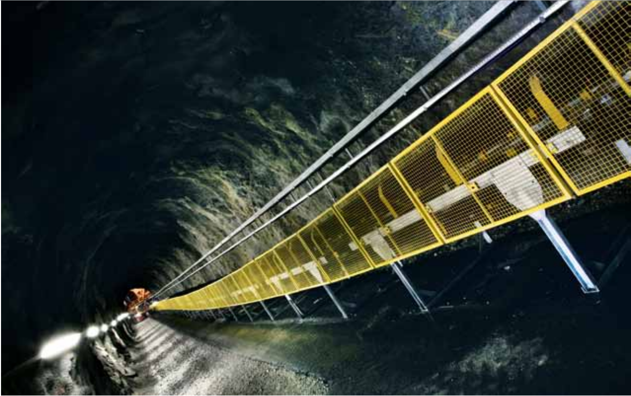
Conveyer belt for raw materials, from quarry to plant, Robilante (CN) – Italy
